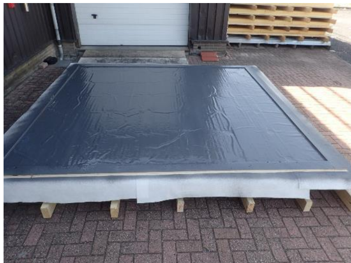
Photo 6 The coating has been applied and the test specimen is ready for testing.
